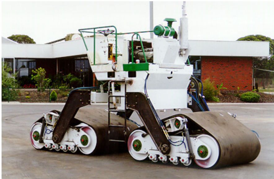
Figure 1.9 A roller built in accordance with HIPAC specifications (Abd El Halim, 2004).
