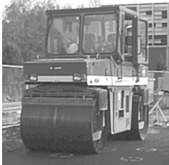
Figure 1.7 A static or vibratory steel wheel tandem roller.
