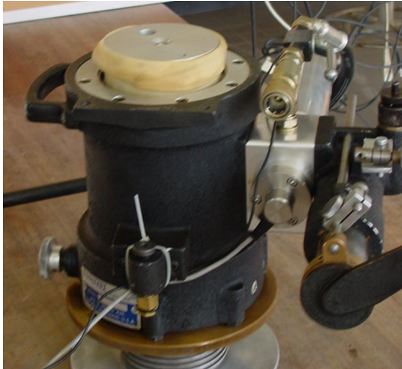
Figure 3.6 The assembled modification (cylinder) in between the standard HSM components.
