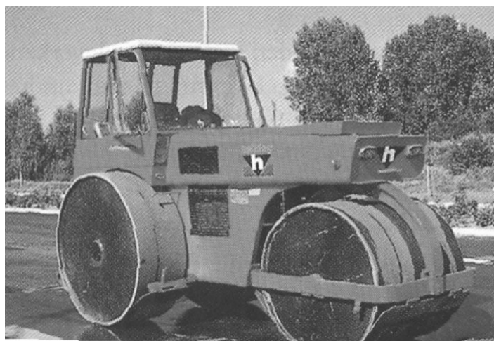
Figure 1.6 A three wheel static steel roller (VBW, 2000).
